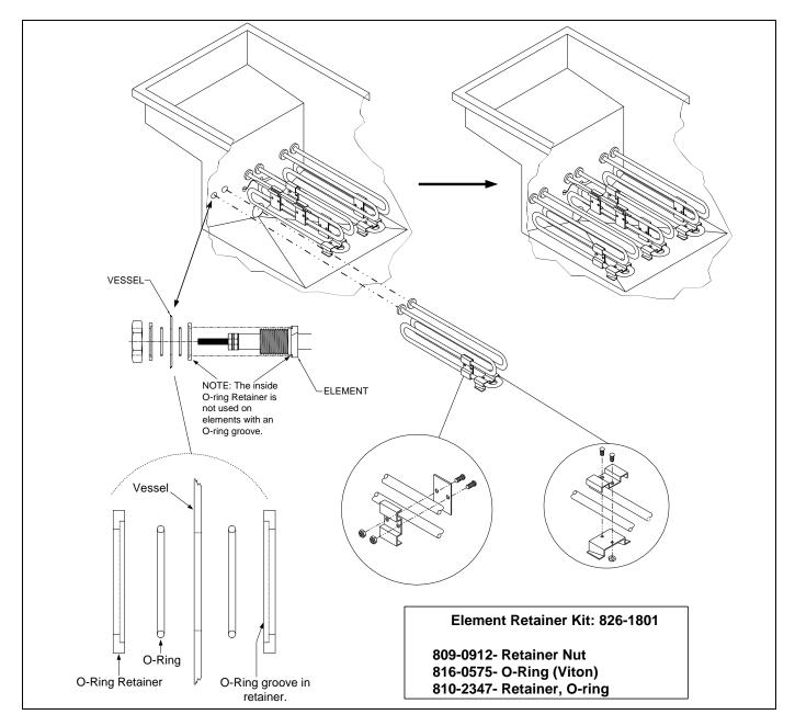
When installing heating elements, assemble O-rings and retainers in the order shown above. Ensure the grooves of the O-ring retainers are facing the O-rings (see illustration). Remove element supports from the old element and install on the new element as illustrated. Ensure all mounting brackets, including probe and high-limit brackets, are properly attached. Questions? Call 1-800-551-8633 for service.
